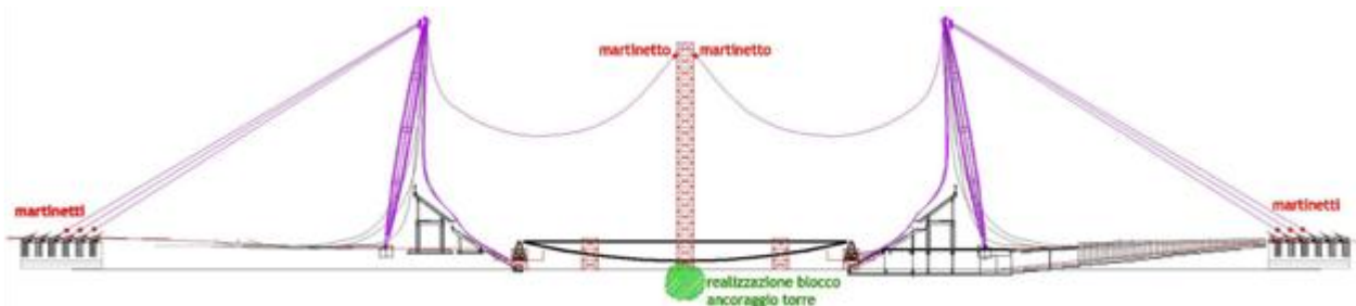
Figure 22: Movement of the main columns until they reach an angle of 14^\circ from the vertical position
