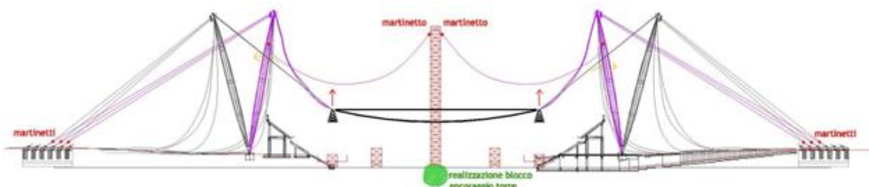
Figure 23: Lifting of the main columns and the main trusses
