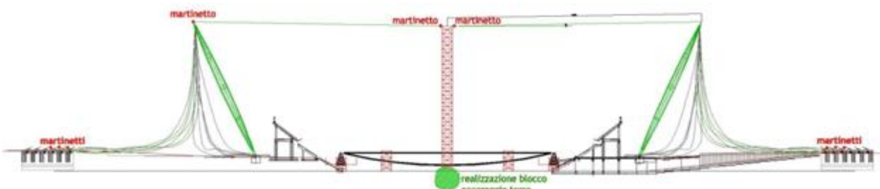
Figure 21: Lifting of the main columns until they reach the vertical position
