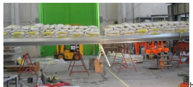
Figure 11: a) Cellular box of steel sheets, b) Experimental tests on cellular box
