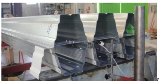
Figure 11: a) Cellular box of steel sheets, b) Experimental tests on cellular box
