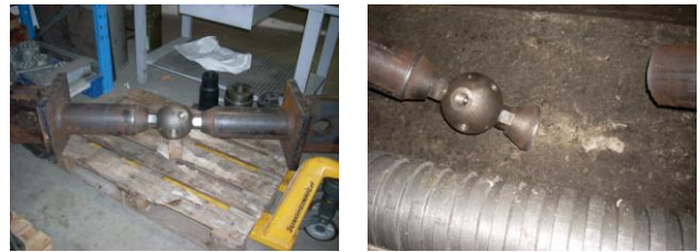
Fig. 6 Resistance test of a node performed on a laboratory
