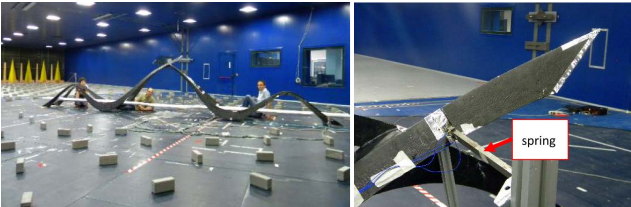
Fig. 3. On the left, 1:50 scale model in wind tunnel: smooth and turbulent flow conditions; on the right, elastic cantilever extension.
