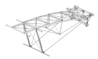
The aerodynamic behavior of the roof has been tested in London RWDI wind tunnel. Innovative and recently proposed techniques have been adopted to perform dynamic analyses under wind action. This allowed static corrections obtained from appropriate pressure distributions, called Proper Skin Modes (PSMs) [2]; thanks to this technique, it has been possible to easily obtain the structural response, without substantial overhead on the structural engineer.
