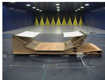
Figure 12. Aeroelastic model for the Braga Stadium
