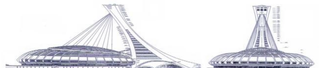
Figure 7 Montreal Olympic Stadium - A cable stayed roof solution
