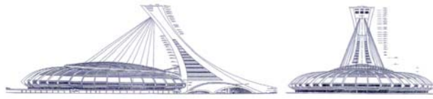
Figure 1 Montreal Olympic Stadium - A cable stayed roof solution
