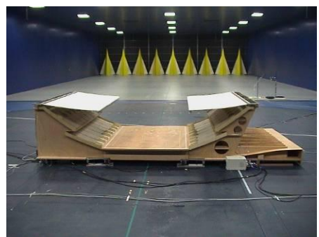
Figure 12. Aeroelastic model for the Braga Stadium
