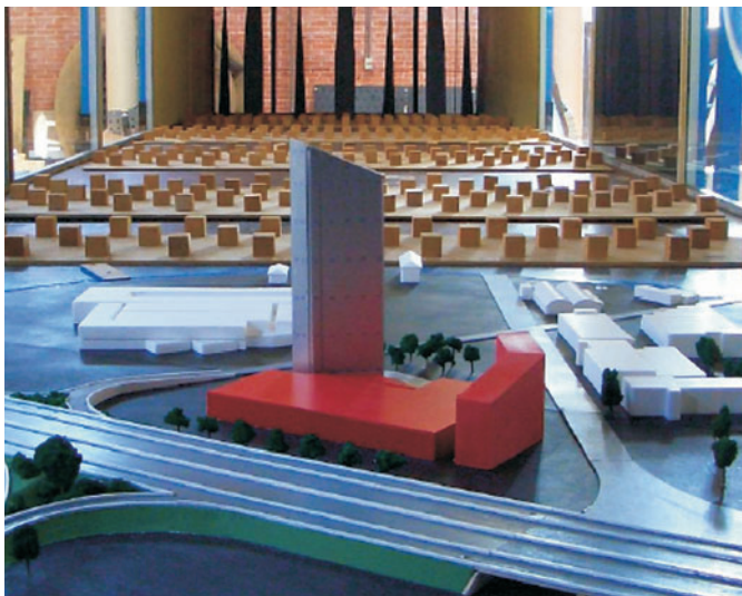
Fig. 18. Wind tunnel test for the Unipol Tower of Bologna
