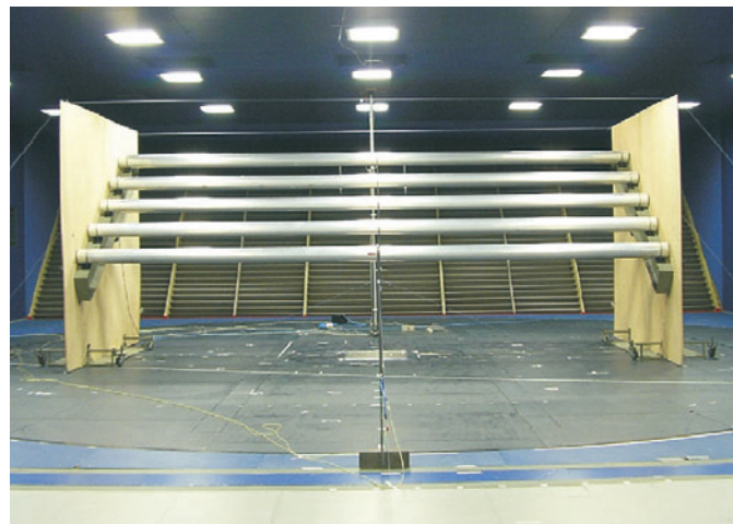
Fig. 19. Wind tunnel test on aeroelastic models for the new city hall of Bologna
