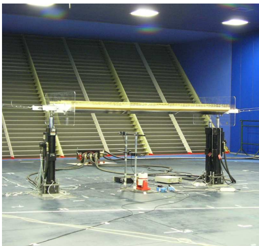
Fig. 21: Experimental deck model (Adige River Bridge- 330m central span)
