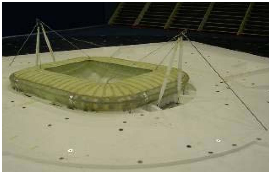
Fig.27. New Juventus Stadium in Turin: example of rigid pressure model [131]
