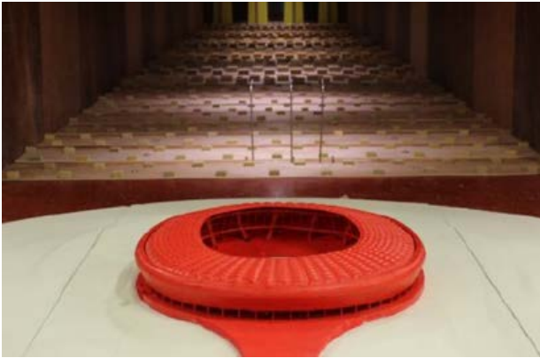
Figure 10-a: Scaled model in the wind tunnel
